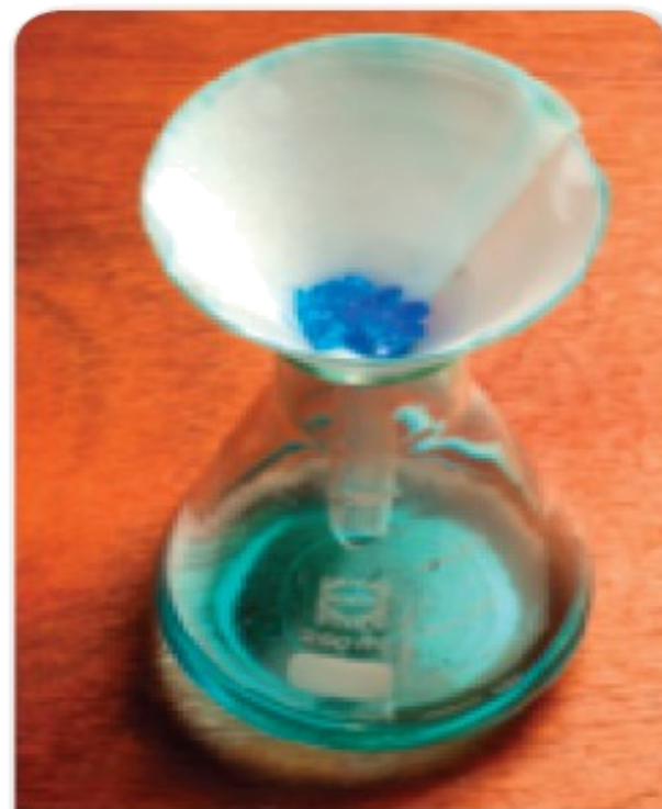
■ Figure 3.13 As the mixture passes through the filter, the solids remain in the filter, while the filtrate (the remaining liquid) is collected in the beaker.
